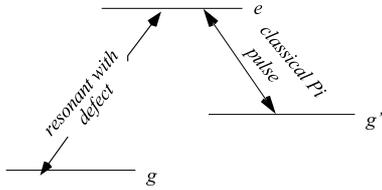
**Fig. 2.** The atomic system consideration. The transition  $|g\rangle \rightarrow |e\rangle$  is resonant with the defect frequency whereas the  $|e\rangle \rightarrow |g'\rangle$  undergoes a  $\Pi$  rotation just before the atoms exit the crystal. The latter is possible through the coupling with an external laser field injected in the crystal through a properly engineered line defect.
